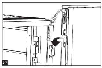
Attach the grounding cable of each rear door to the grounding points of the extension frame as shown. (Use the screws and washers removed in step 2-1.)
